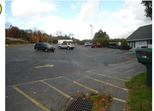
**1** **POROUS PAVEMENT:** Sections of porous pavement could capture and infiltrate a large portion of parking lot runoff. Reducing runoff from the parking lot helps reduce sediment and nutrient loadings to local waterways, enhancing water quality.
